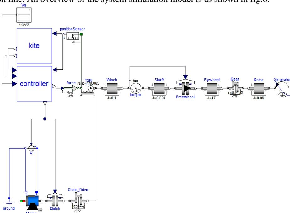
**Fig.6:** Illustration of the proposed AWEs simulation model
